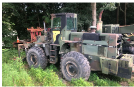
International M 10A loader w/forks and 10,000lb. lift capacity
