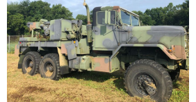
5 ton wrecker w/20,000 lift capacity, all wheel drive diesel
