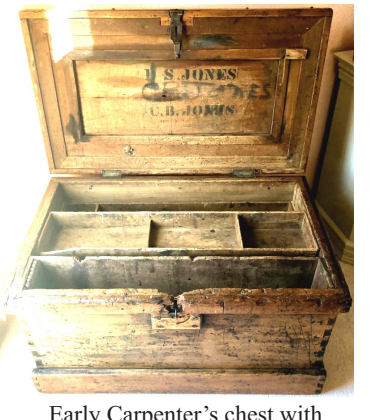
Early Carpenter's chest with exposed dovetails
