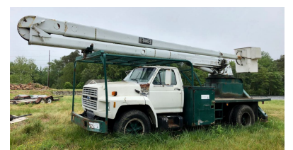
53 ft. Hi Ranger Bucket Truck Single man bucket, in good operating condition, mounted on a 1994 Ford F 700 truck, 6 sp. man. trans., Cummins Diesel w/140,000± miles
